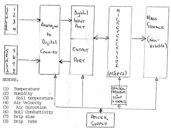
Once a month the Mass storage device is exchanged and then transported to the data processor in Canberra. This will make the data readible on a printed sheet; or format the data on to some other storage medium so it can be used elsewhere.
