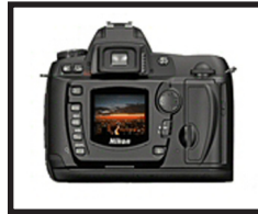
Figure 8: Fixed LCD on a digital SLR - used to view images only after they are saved to memory.
