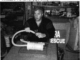
This provides a robust light-weight, water-tight container for the chemical contents. A coarse stainless steel strainer fixed in position covers the inside of the entry and exit ports.
