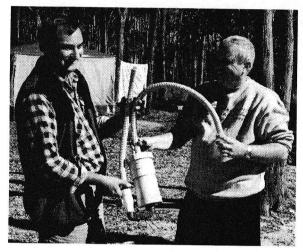
The unit was easy to transport despite a temporary belt attachment, which proved troublesome. This initial design had an intake tube to permit snorkelling. It was quickly found to be a hindrance as the end of the tube was often blocked on the back of the overalls. The next version will have a strainer intake, which cannot be sealed off accidentally.
