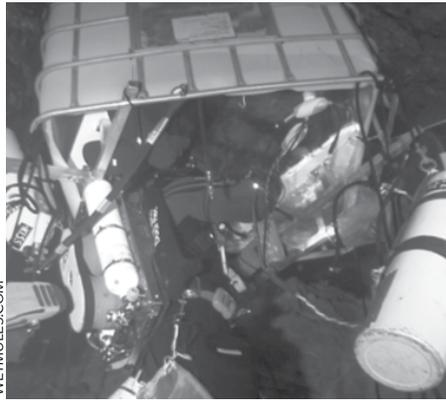
A support diver under the 28m habitat helps get the push diver settled in. Surface supplied heating cable can be seen in the right-foreground.
