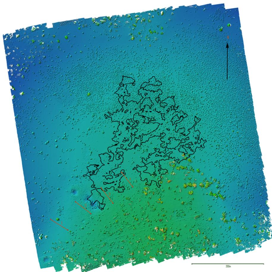
Digital Elevation Model (DEM) of the area over Witches Cave, courtesy of Daniel Burt, with overlay of cave map traced from Alan Pryke's knz file, and seismic lines 1 to 4 in red
