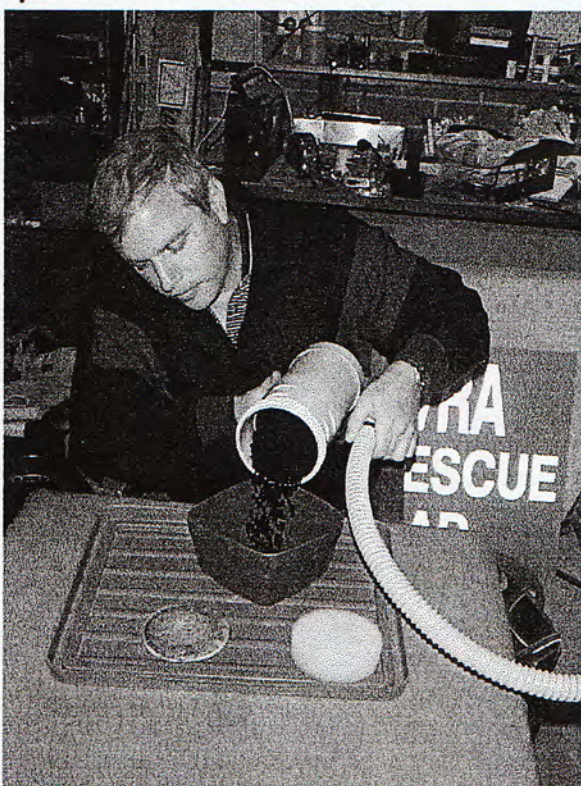
Dave has removed the spacer filter and HEPA filter to empty the activated carbon.
