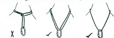
Single or double looped slings give better loading angles and creates undue stress due to the wide angle produced.
