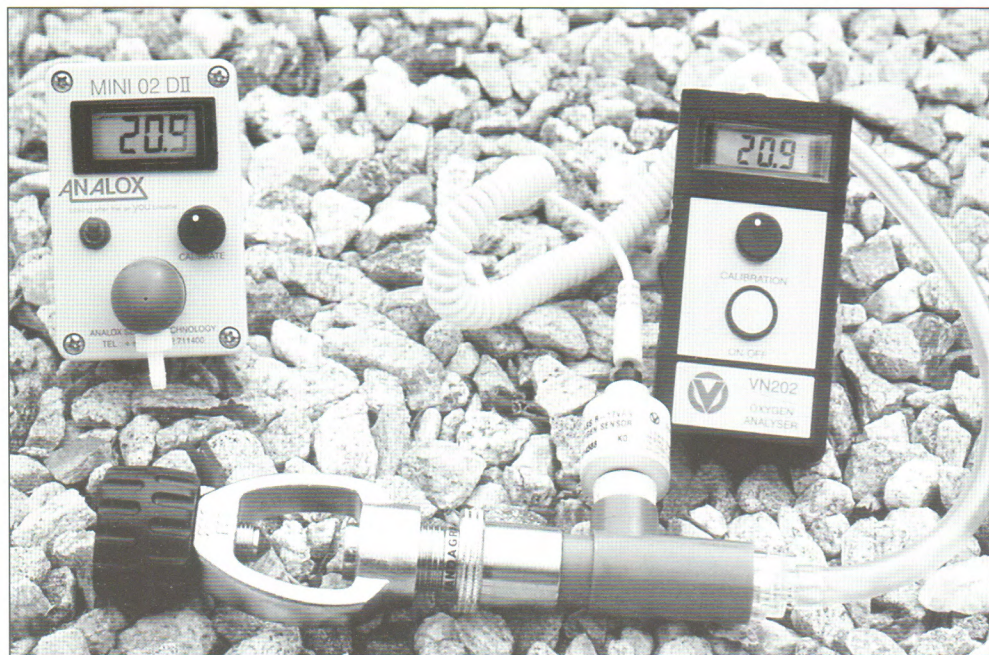
While electronics cases may appear similar, the method of getting the gas to the sensor can be markedly different.
