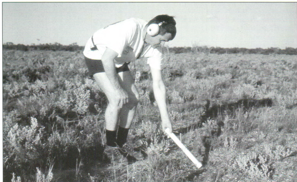
Locating the 45 degree point for depth measurement.
