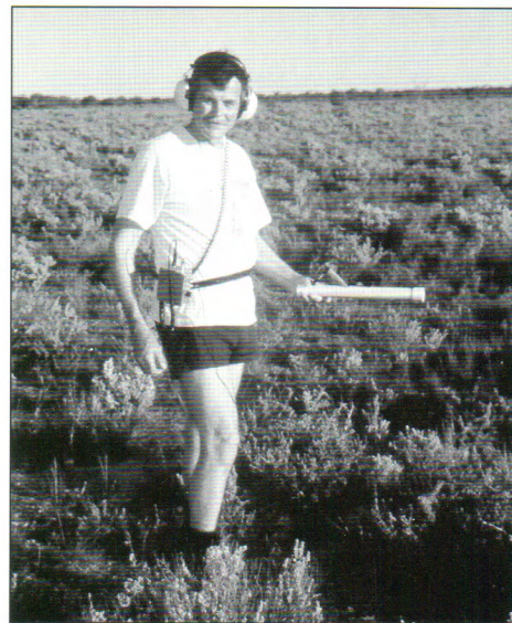
Using the receiver coil to locate ground zero.
