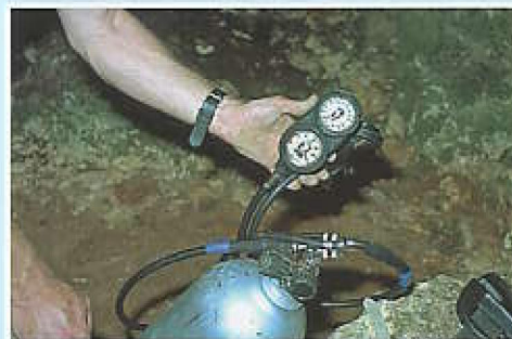
Tanks were over-filled, leading to issues with burst disks and regulator hoses. One high pressure hose and one scuba feed hose blew on the push dive. In anticipation of such problems, spanners and plugs were taken and these problems fixed on the run during the dive.
