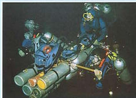
A broom handle was put through the front of the sled and 3 divers worked together to push the whole arrangement along. Controlling buoyancy was a major problem, and progress was often slow.
