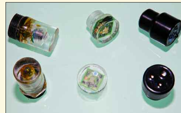
[Photo 2] Slave sensors from left to right: homemade for an Ikelite wet connector, Heinrichs Weikamp RSU-N, triggerfish
