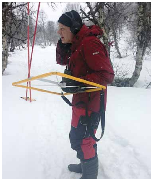
The original discoverer of the cave, Bo, doing precise radiolocation of the divers underground (Courtesy of Expedition Bjurälven)
