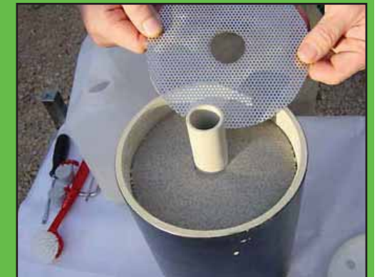
Packing the RB80 scrubber. A common design and very simple to homebuild.
