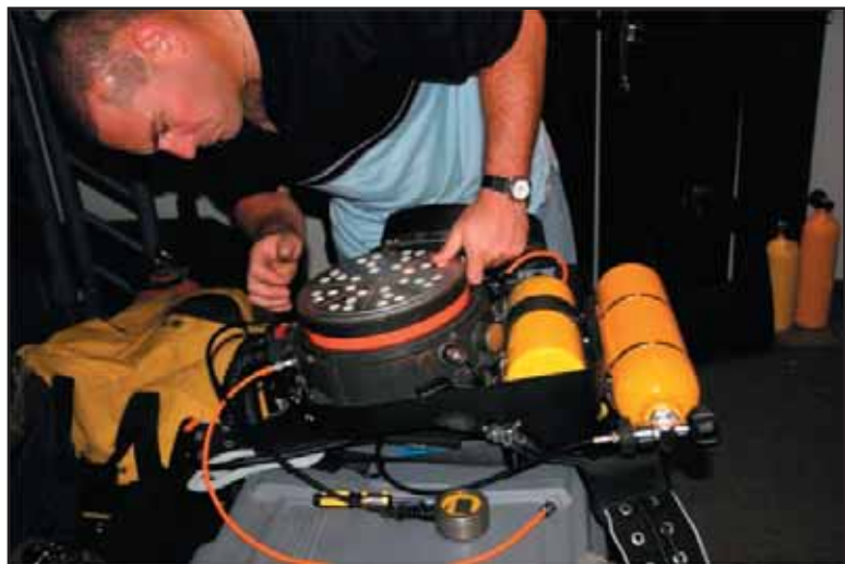
Left: Here you can see the electronics port on the side of the centre section and the scrubber canister itself. A few last minute checks for the electronic unit from Kane Willcox prior to going in the pot.
