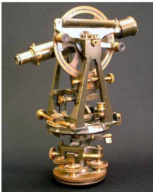
Troughton and Simms theodolite Ca 1880, similar to the type of theodolite that Turner would have used.
