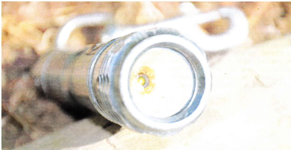
The now worthless TOVATEC backup dive torch, caused by the “Rapid Disassembly” of a battery
