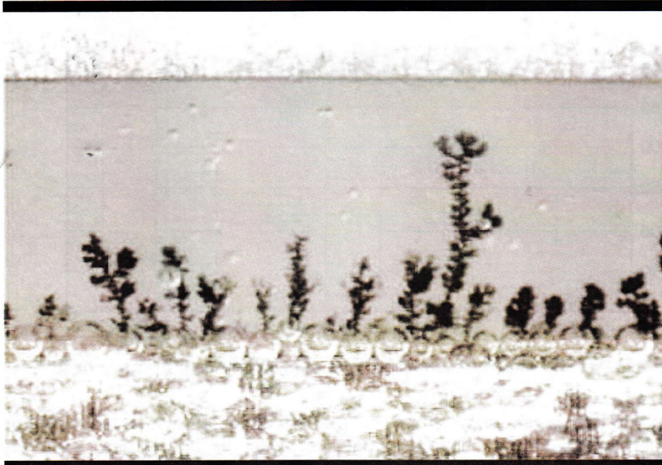
Microscopic Lithium dendrites growing out from the anode, toward the cathode
