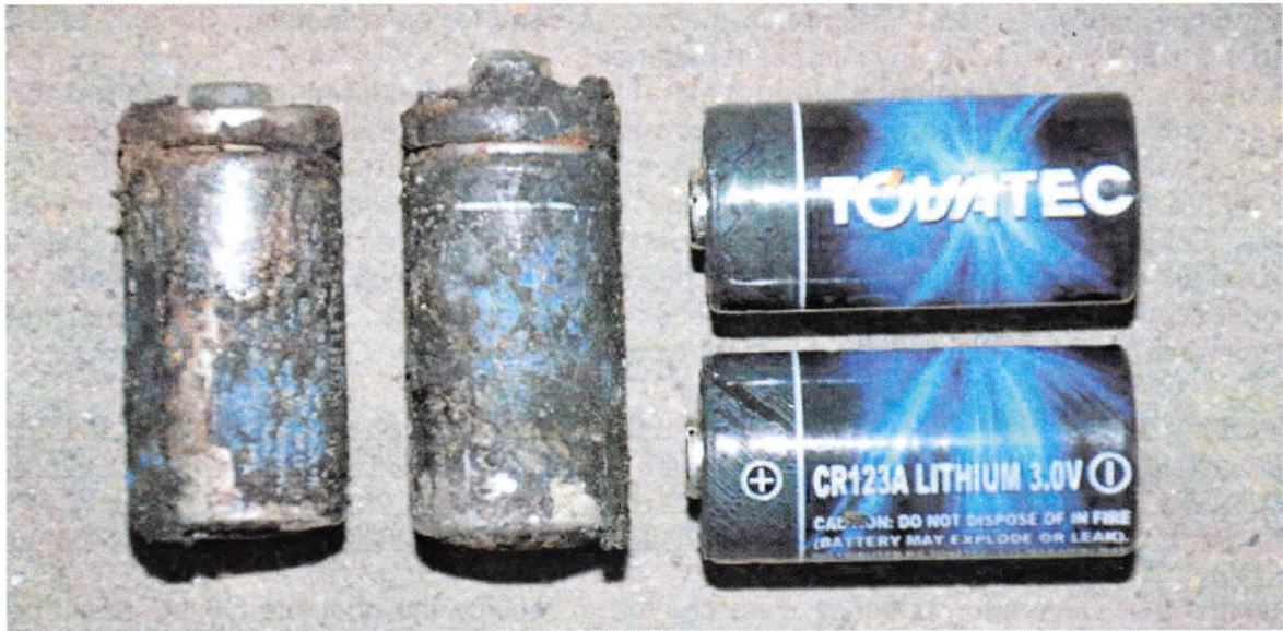
The two destroyed batteries, with two others bought at the same time – note one is considerably swollen.
