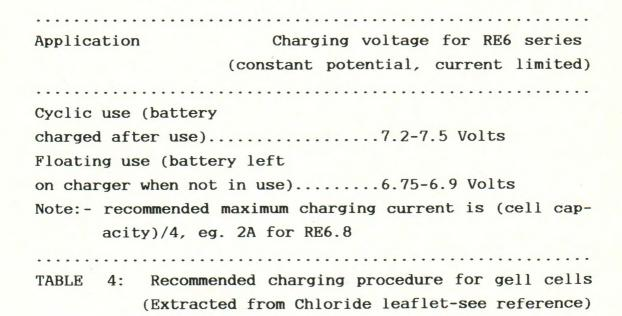
One of the best options is to build your own charger, this is not as difficult as you may think. Integrated circuit voltage regulators are readily available and with the addition of a few external components an excellent charger can be built (even by the novice, with a little help!). A convenient circuit to follow is depicted in SOUTHERN CAVER 8 JANUARY 1987
