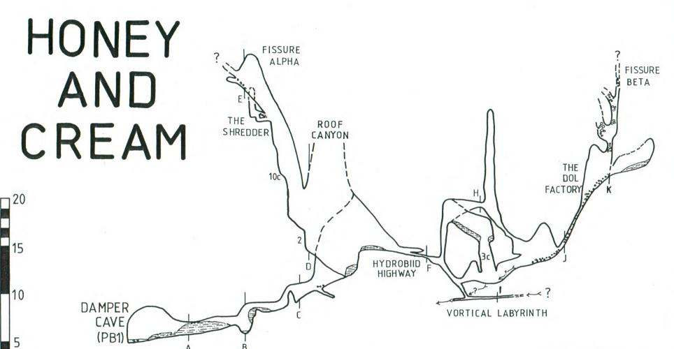
DEVELOPED LONGITUDINAL SECTION VERTICAL EXAGGERATED BY 2.5 TIMES
