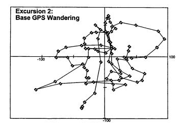
The graph (left) shows the wanderings of the Base GPS over the time that it was operating. The standard deviation of these positions is 56.6 m. This plot shows the effects of Selective Availability quite clearly and shows that a spot reading, or any reading averaged over a few minutes could easily be 100 m off the true position.
