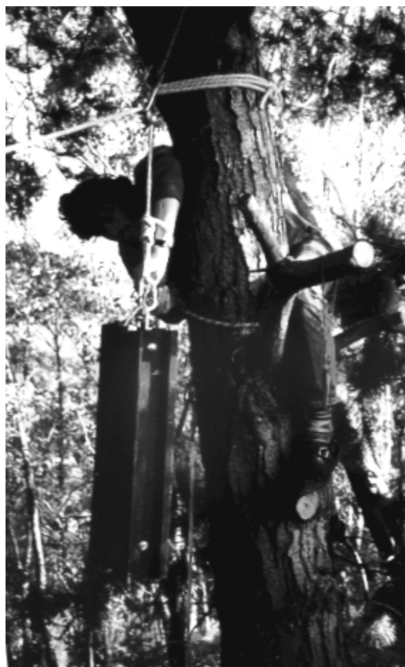
Hugh (up the convenient Drop-Testing tree), securing 'Buster' (3*27 kg pieces of railway line) to a safety and stringette, prior to removing the haul rope.
