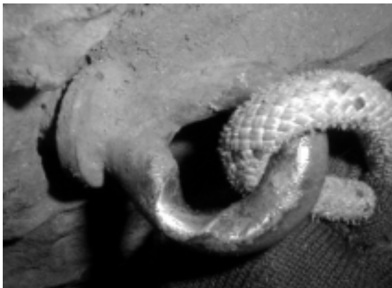
Pitch 5-Eyebolt showing the wear from rope pull-throughs.
