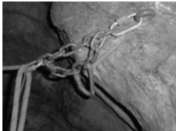
Pitch 6-a 'rats nest' of rigging tat attached to the Eyebolt. Note the deep grooves in the limestone below the bolt.
