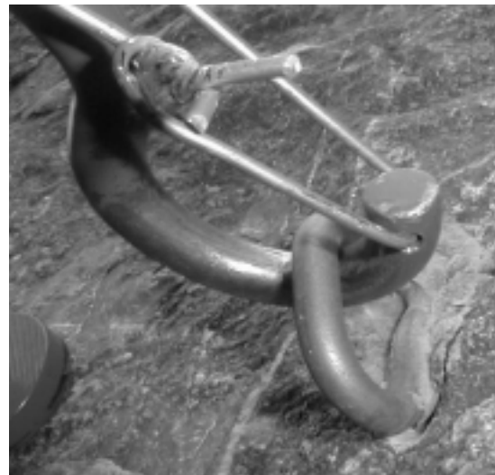
Bolt 5 under test with 14 kN force applied. Note that the lower part of the eye has flexed away from the rock. Note also the 'wire gate' used to strengthen the 'testers hook'. the force that 99.87% of the population will exceed. Ideally this 3-sigma limit should be ~20 kN or more.
