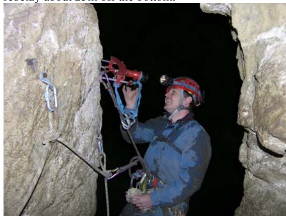
Gavin testing a P-hanger in Goodbye Chamber (it passed!). Photo Alan Jackson
