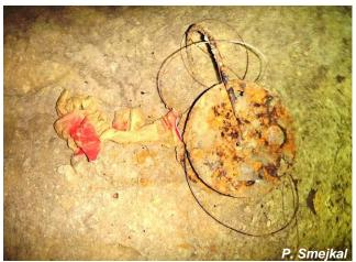
Corroded cable in Telephone Room.
