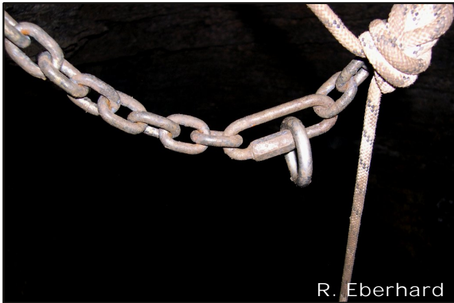
Plate 3. Fixed rigging in Ice Tube (December 2012). Note potential for three way loading of maillon.
