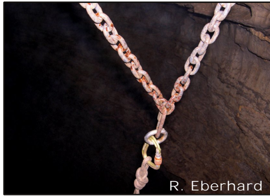
Plate 1. Fixed rigging in Ice Tube (December 2012). Note evidence of corrosion to chain.
