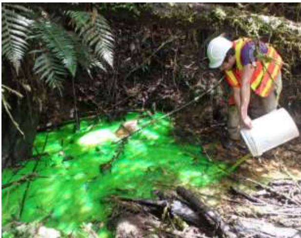
Photo 1. Jeffrey Prado inserting fluorescein dye into the SF-267 stream sink, 15 November 2014
