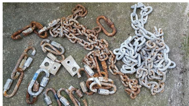
The hardware removed from Ice Tube and why we don't use non-stainless material in permanent cave rigging.
