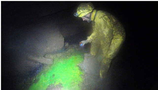
Pax releases a carefully calculated amount of fluorescein in Sesame.
