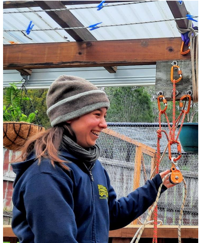
How not to rig a triple load share (missing twists and carabiners undone)! Photo: Gabriel Kinzler
