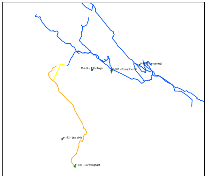
Survey plot, showing Porcupine (blue), the push (yellow), Gormenghast (orange) – loop not closed, 60 m error
