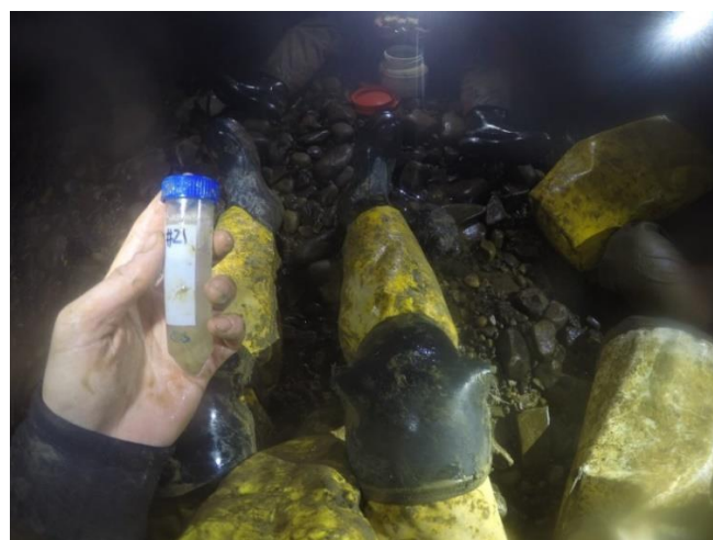
These centrifuge vials were pre-labelled and filled with ethanol, so a GoPro video could record the details
