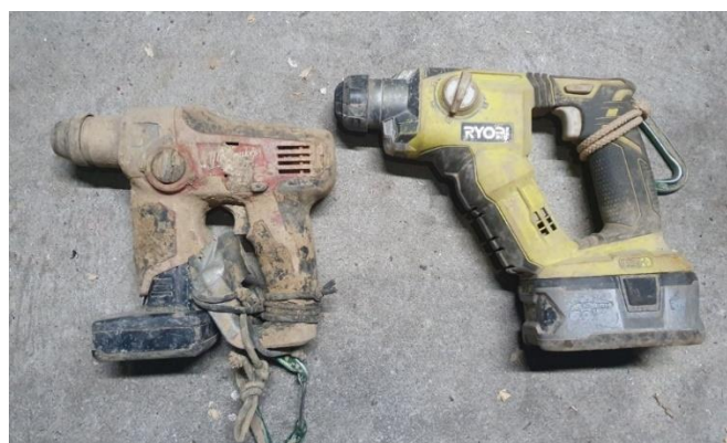
Comparative size of 12V Milwaukee (left) and 18V Ryobi (right)
