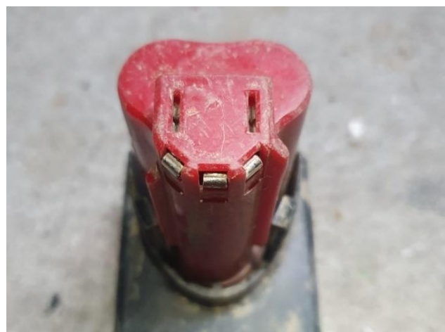
12 V Milwaukee battery, terminals anticlockwise from top left are: Positive (Cell 3+), Cell 2+, Cell 1+, Temperature Sensor, Negative (they are actually labelled in tiny, raised lettering).
