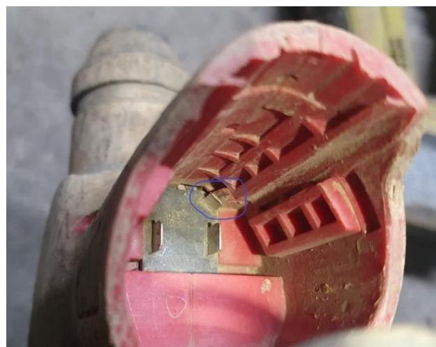
Inside battery socket of 12 V Milwaukee drill – the temperature sensor terminal is circled.
