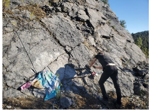
The test site and setup in the Junee Quarry. Left to right: screw and hanger on (under a towel to control small projectiles at failure), chain running from screw to load cell, load cell, welded angle bracket and Hilti load tester, and muscle.
