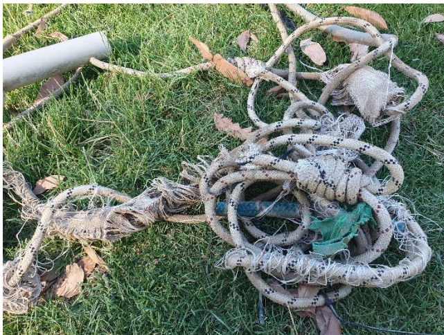
The rope used for anchors – garden hose rope protectors survived ok, but the woven ones not so much (the rope wasn't damaged though)
