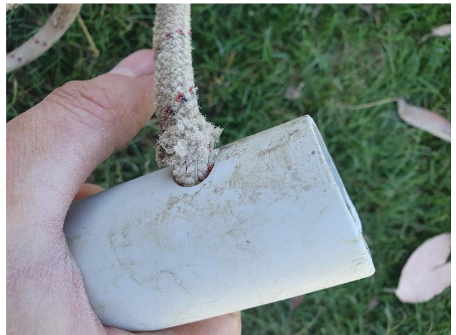
Core shot caused by abrasion of rung
