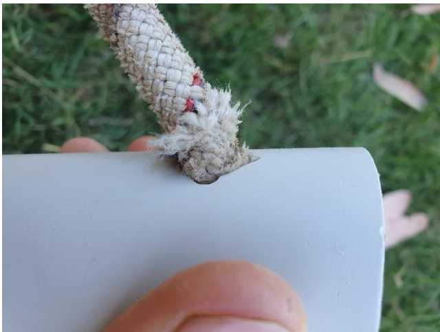
Sheath abrasion at split section of rung
