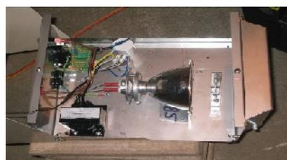
Figure 3 – a light driver (with cover removed) showing lamp housing, infra- red filter and electrical components.
